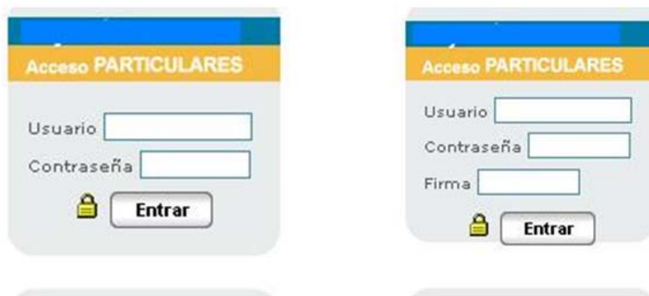
Image 4: Example of injection of a fraudulent form field into a bank's legitimate website.
